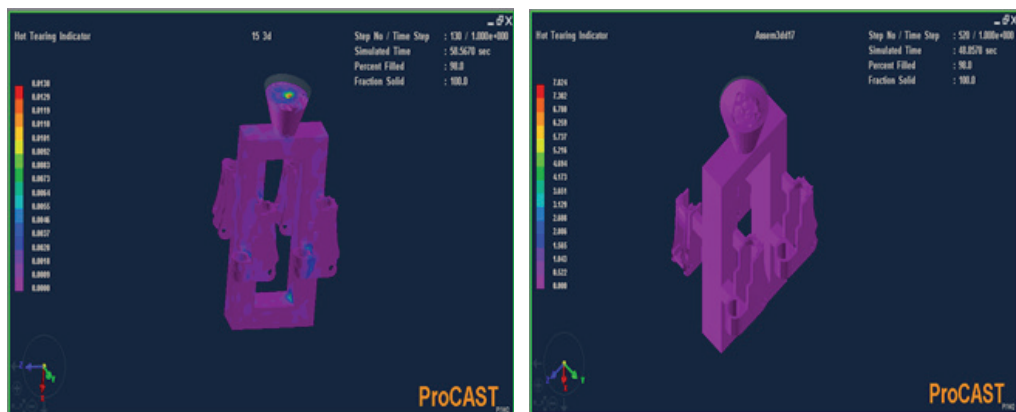
Figure 14. Result of hot tearing of 15 mm gate length with in 1580 °C pouring temperature; result of hot tearing of 17 mm gate length with in 1630 °C pouring temperature
