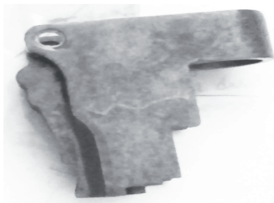
Figure 5. Process and results of magnetic particle inspection method, result shows there is some void/crack/hot tearing
