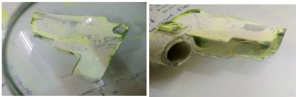
Figure 4. Result of liquid Penetrant inspection, casting defect hot tearing/crack
