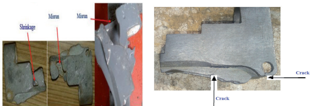
Figure 3. Visual testing, casting defects (misrun and shrinkage porosity) and crack
